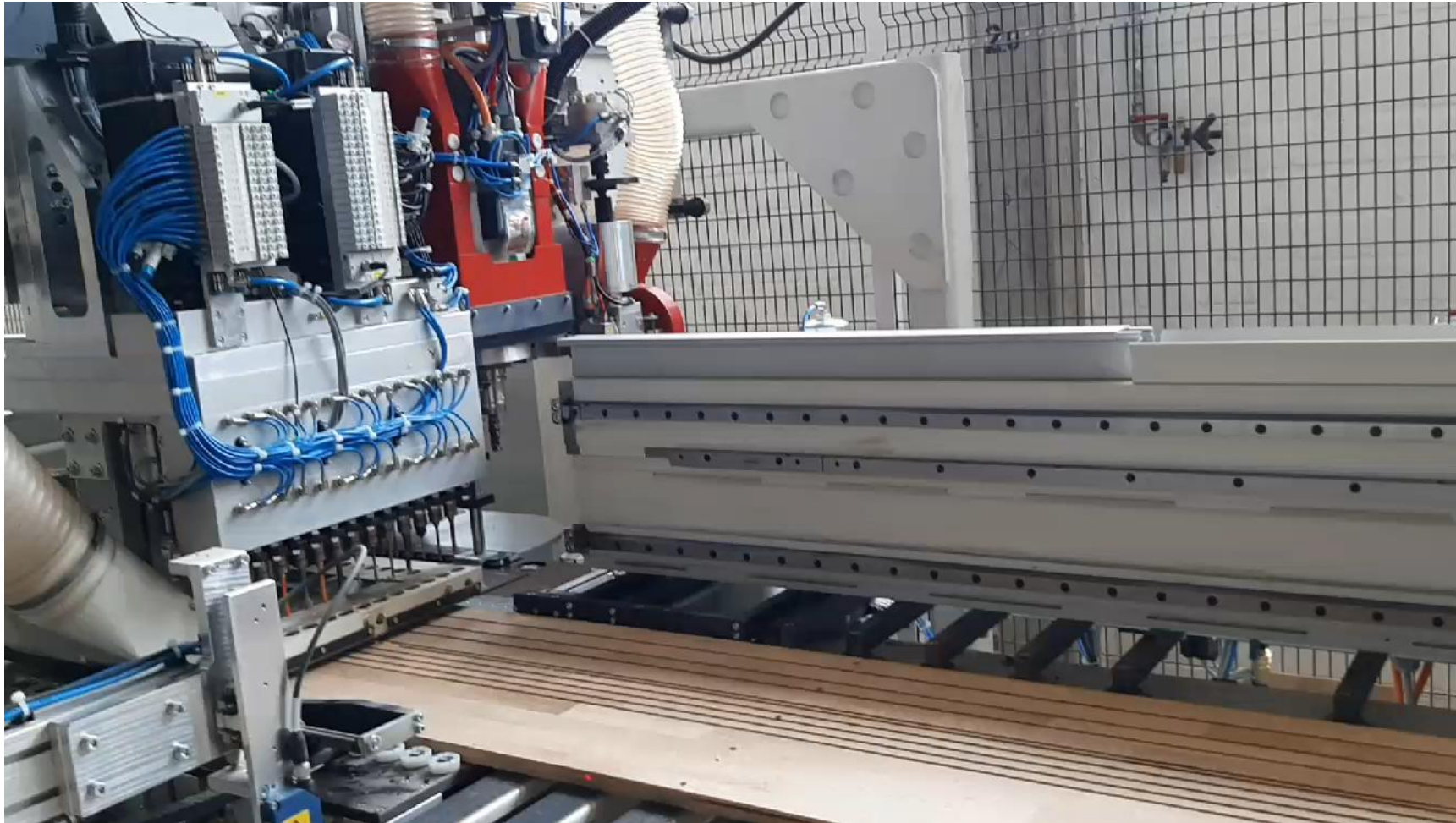
Groove saws with Compact module – 6mm wide and 9mm deep grooves in beech
