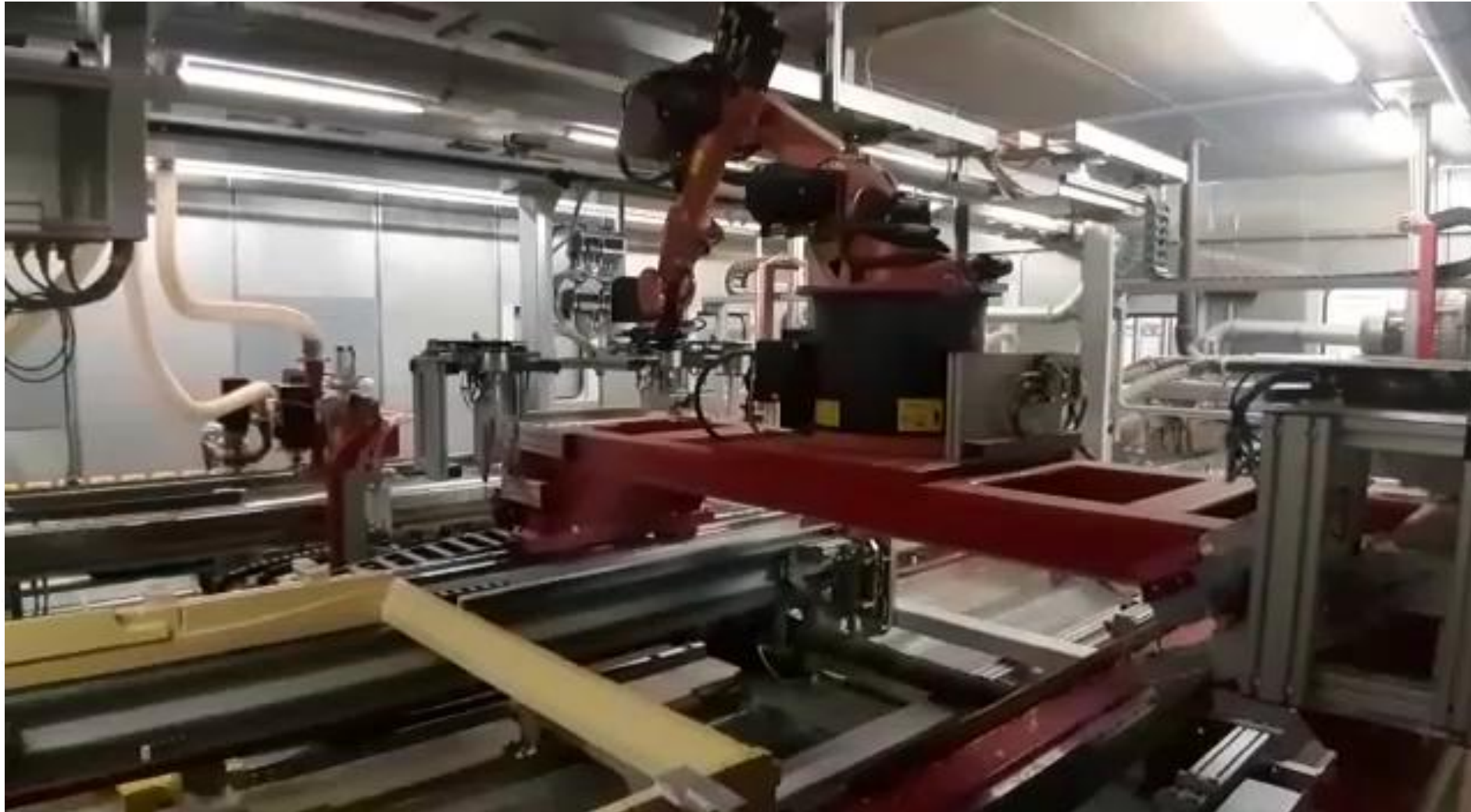
Milling and drilling with robots KUKA KR16
