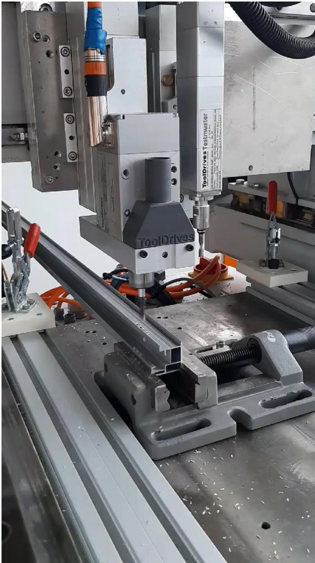
Milling vs drilling 8mm holes in ALU
