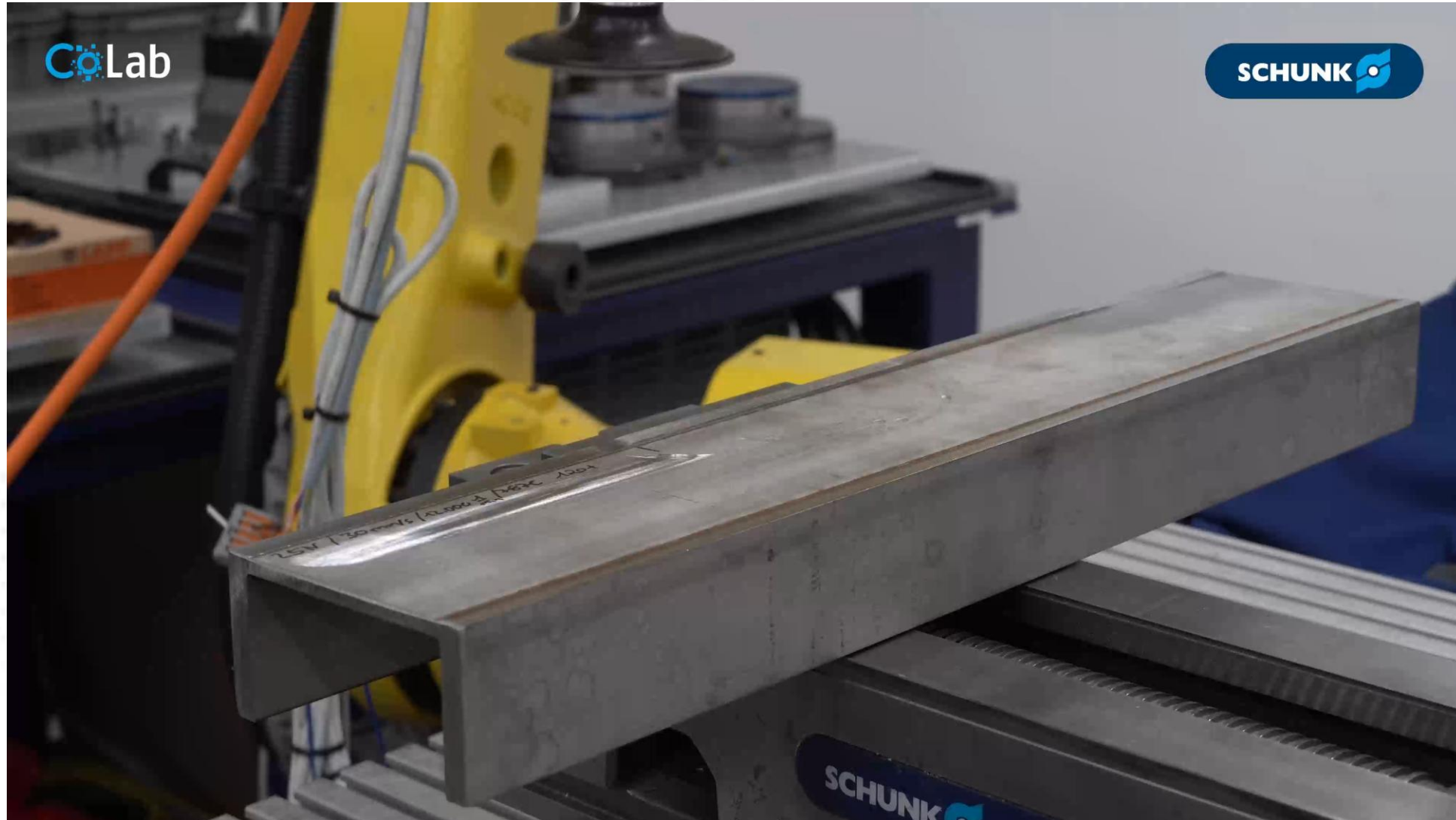
Robotics Grinding Welds with Fanuc - Schunk CoLab
