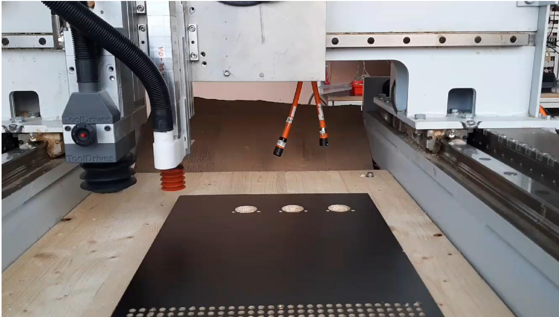
Drilling: 35mm Pot Tape Holes with Suction
