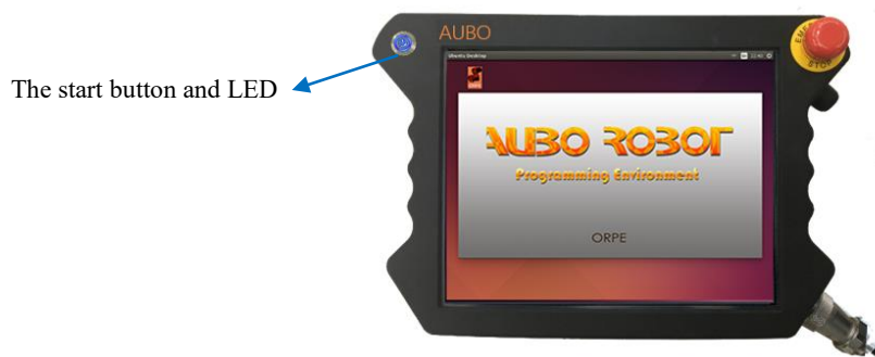
Figure 9-2 the start button and LED indicator
