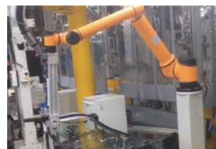
Gluing of vehicle windows
