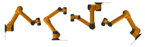
Figure 6-5 Diagram of different installation poses
