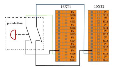
Figure 8-12 Force control enable input
