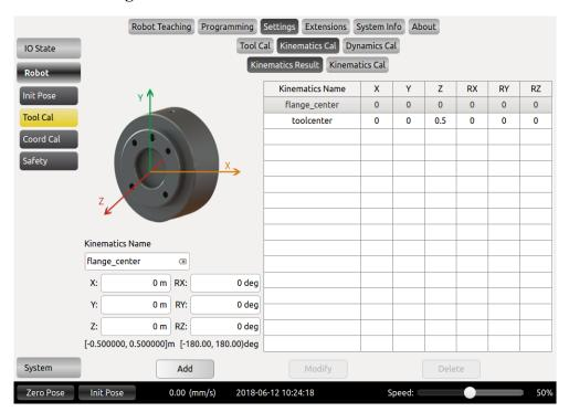
Figure 10-36 Tool Kinematics Settings
