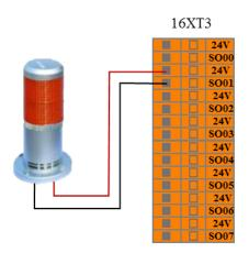
Figure 8-17 Figure robot moving output connection
