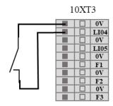
Figure 8-33 Remote start up connection
