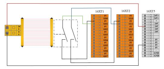
Figure 8-6 Safeguard stop input (Internal Power Supply)
