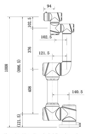
$Figure\ 6\mbox{-}1\ AUBO-i5\ mechanical\ dimensions,\ unit:\ mm$
