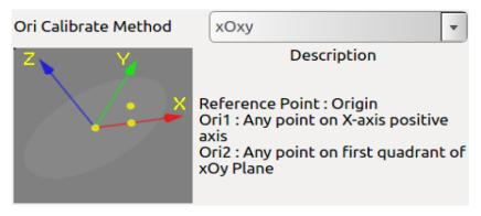
Figure 10-30 xOxy type calibration method
