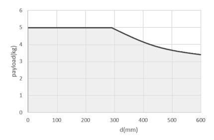
Payload of wrist has shown above, in which d-axis represent the center of gravity offset which is the distance between end-effector flange focus and tool focus.
