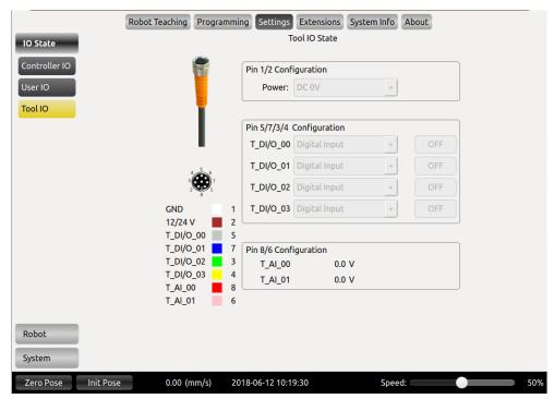
Figure 10-26 Tool I/O panel
