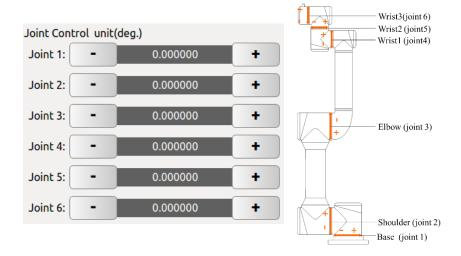
Figure 10-17 Illustration of joint control.
