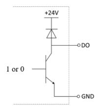
Figure 8-24 DO connect GND
