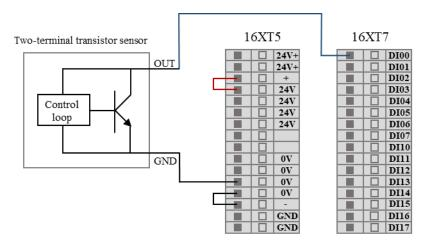
Figure 8-26 DI connect to two-terminal sensor
