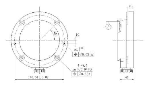
Figure 6-6: Mounting whole size of the manipulator base.
