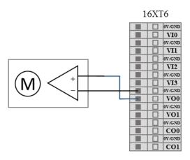
Figure 8-29 Analog voltage output connect drive device
