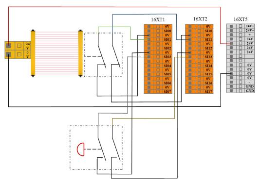
Figure 8-9 Safeguard stop Resert Input connection (Internal power supply)
