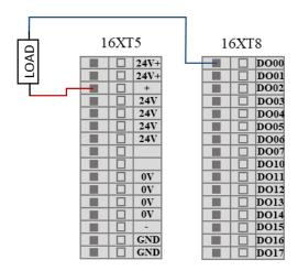
Figure 8-27 DO terminal connect external load
