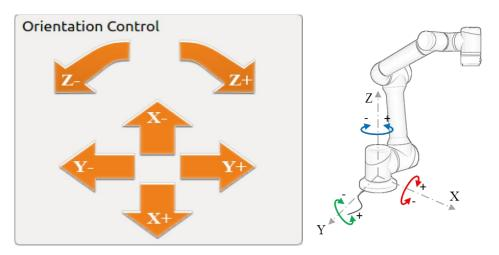
Figure 10-15 Orientation Control (base)
