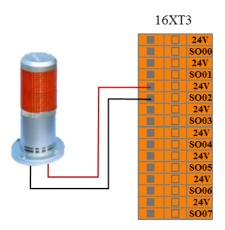
Figure 8-18 robot not stopping output connection
