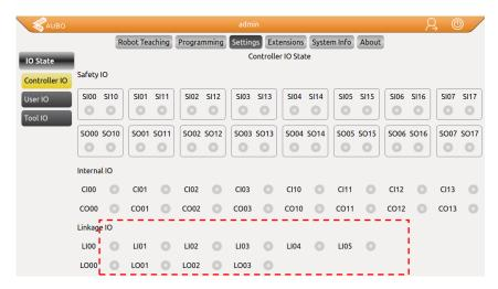
Figure 7-9 AUBOPE software "Settings" tag, Linkage IO status
