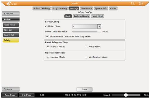
Figure 7-7 AUBOPE software "Setting" tag
