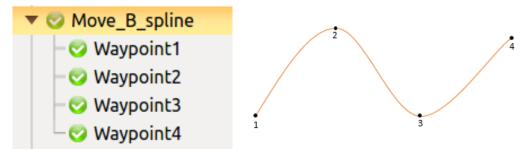
Figure 11-21 B-spline curve
