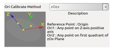
Figure 10-32 zOzx type calibration method
