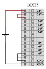
Figure 8-3 external power supply schematic
