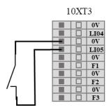
Figure 8-34 Remote shutdown connection
