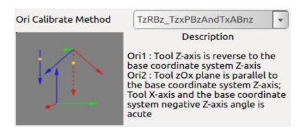
Figure 10-35 TzRBz\_TzxPBzAndTxABnz type calibration method
