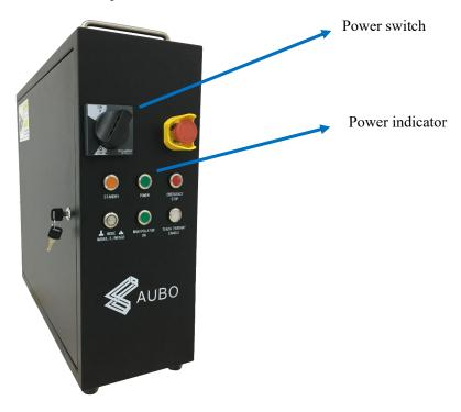
Figure 9-1 Control box side panel
