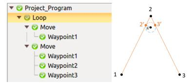
Figure 11-20 blending radius motion track
