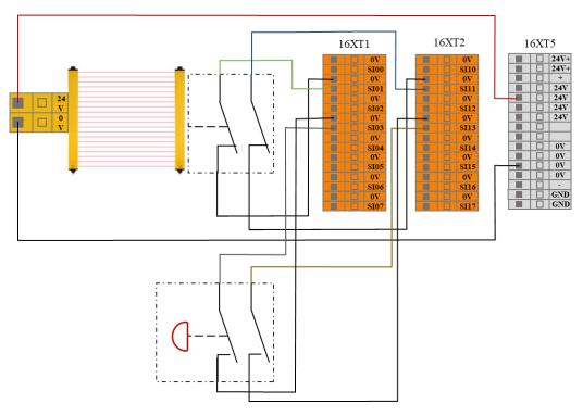
Figure 8-7 Safeguard stop input (Internal Power Supply)
