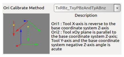
Figure 10-33 TxRBz TxyPBzAndTyABnz type calibration method
