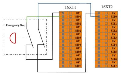
Figure 8-5 External emergency stop input
