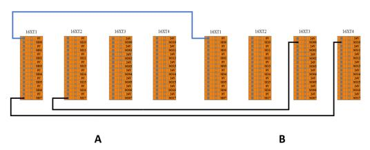
Figure 8-14 system stop input connection (From B to A)
