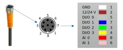
Figure 8-36 Robot Tool I/O wiring order
