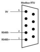
Figure 8-1 Modbus pin description
