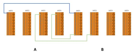
Figure 8-13 system stop input connection (From A to B)
