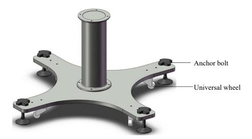
Figure 6-3 Diagram of manipulator base structure
