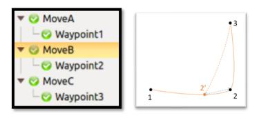
Figure 11-22 Arrival Ahead – Distance/Time Trajectory Example
