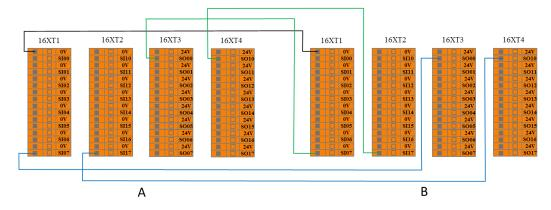
Figure 8-15 **Prohibited** system stop input connection
