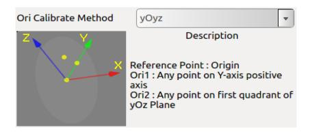
Figure 10-31 yOyz type calibration method
