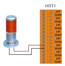
Figure 8-21 System error output connection
