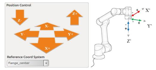
Figure 10-10 Position control (Flange center)
