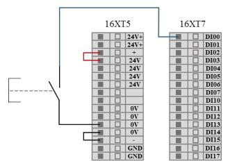
Figure 8-25 DI terminal connection button switch schematic
