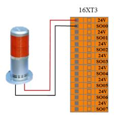
Figure 8-16 robot emergency stop output connection
