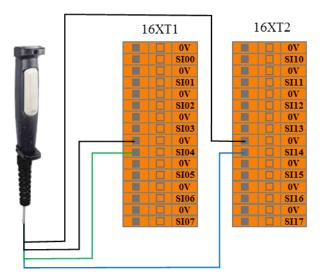
Figure 8-10 Enabling device input connection
