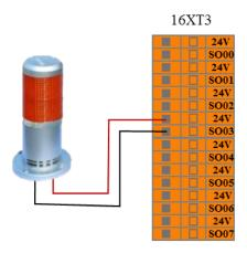
Figure 8-19 reduced mode output connection
