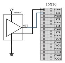
Figure 8-30 Analog voltage input connect to sensor
